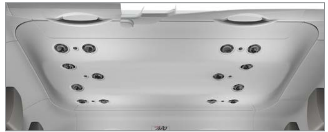
Optional headliner with LED lights and adjustable air vents.
