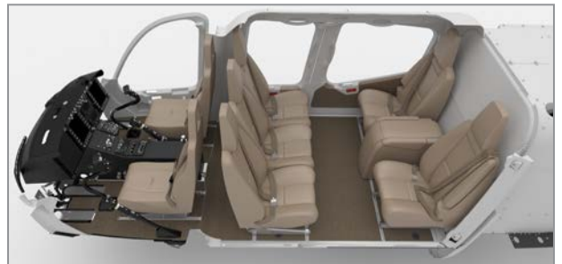
Five place club seating with a row of two 21.5" seats separated by a center console facing a row of three 18.5" seats.
